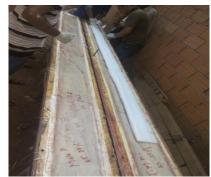
Fig 10: Filling airfoil mould with composite mixture
