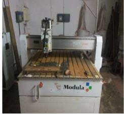
Fig 2: CNC router machine
