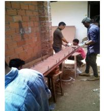
Fig 11: fastening male and female parts for curing
